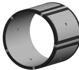
Fig. 3. Virtual textured journal bearing: A smooth bore journal bearing is supplied through the holes with a MR-lubricant. Virtual recesses are created by the magnetic field created in the dark zones. In operation both hydrostatic and hydrodynamic load carrying capacity is generated.
