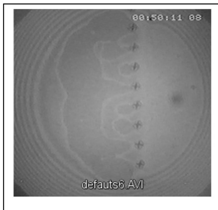
Dewetting of an intercalated lubricant film behind nucleators
